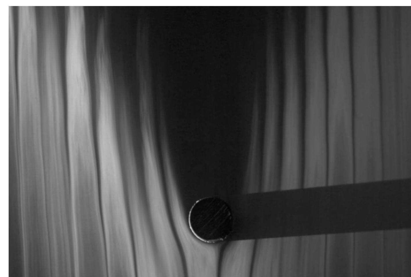
Figure 4. Smoke seeded airflow around 5mm cylinder at 0.35 m/s airflow. Qualitatively shows laminar flow.
