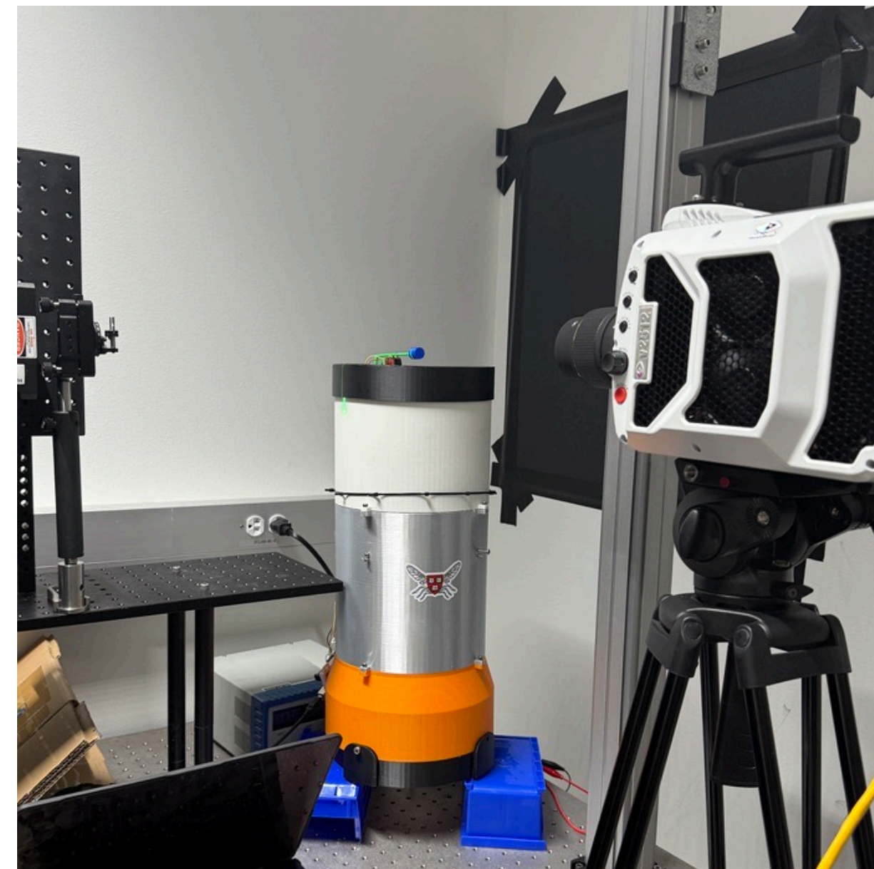
Figure 2. PIV testing setup with high speed camera positioned to view smoke-seeded airflow around the 10mm cylinder.
